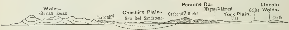
Fig. 5.—SECTION FROM SNOWDON TO THE EAST OF ENGLAND. According to Professor Ramsay.
